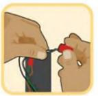
insert the wires into wire nuts.
