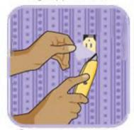
Cut around outlets, replace the plates.
