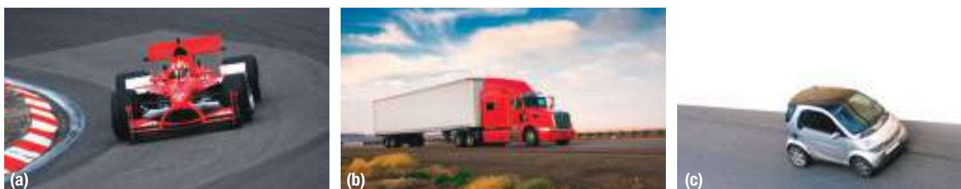
Figure 1 (a) A race car speeds up quickly because it has a small mass and experiences a large net force. (b) A truck accelerates more slowly. Even though a large net force acts on it, the mass is large. (c) A small economy car also accelerates more slowly. It has a small mass and a small applied force.
