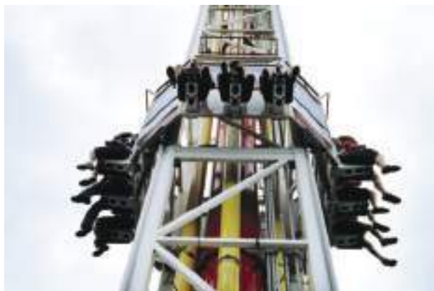
Figure 4 Drop-tower rides use an electromagnetic braking system that is reliable and automatic and has parts that do not wear out.
