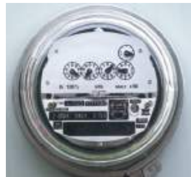
Figure 2 Electricity meters measure the amount of electrical energy used.
