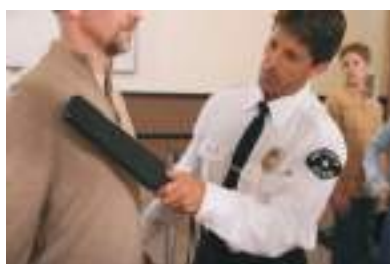
Figure 4 Metal detectors like this one use electromagnetic induction.
