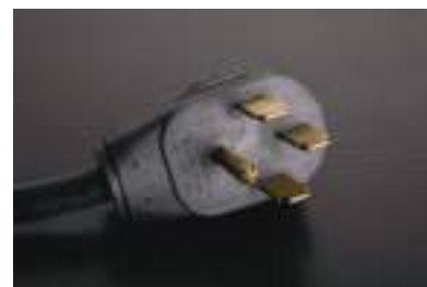
Figure 3 A plug for an electric stove or clothes dryer is designed for a maximum alternating current of 30 A at 240 V. Since it has four prongs, it can also supply 120 V for parts of the appliance that do not require 240 V (such as control circuits).
