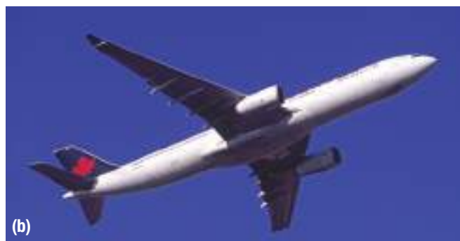
Figure 1 (a) The wings on a propeller plane are perpendicular to the airflow. (b) The wings on modern passenger jets are angled, so the airflow over the wings is smoother. The greater the sweep of the wings, the faster the airplane.
