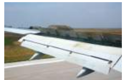
Figure 2 Aerodynamic brakes cause normal vibrations in aircraft.
