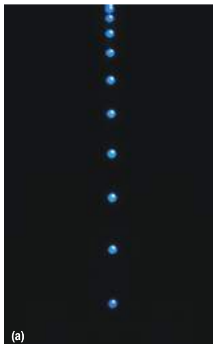
Figure 2 (a) Multi-flash photograph of a ball in free fall starting from rest (b) Multi-flash photograph of a light object with large surface area in free fall. Which object is accelerating? How can you tell?
